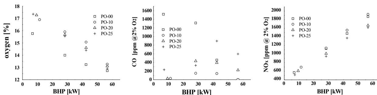
Figure 4. Emissions ( $O_2$ , CO, and  $NO_x$ ) - engine at constant angular speed (2,500 RPM).
