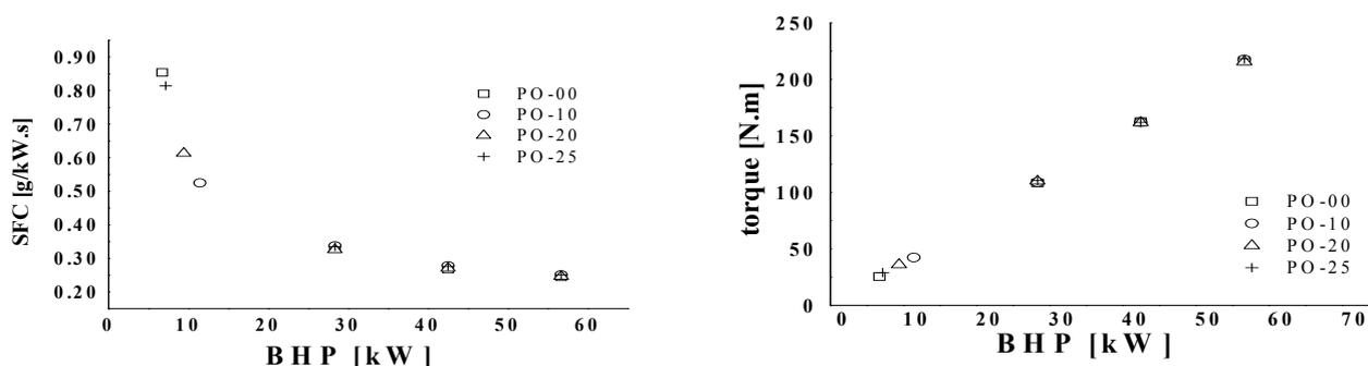
Figure 3. SFC and Torque versus BHP – engine at constant angular speed (2,500 RPM).
