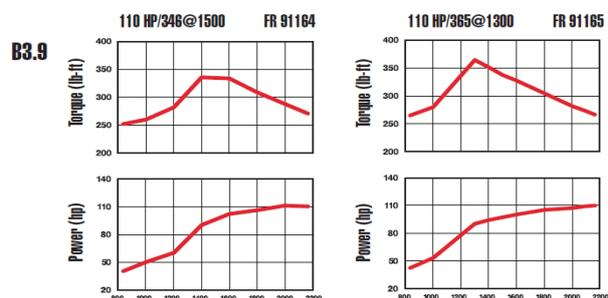
**Figure 2.** Experimental apparatus (setup and dynamometer bench test) for Diesel engine and characteristic curves from the manufacturer (Cummins, 2018).
